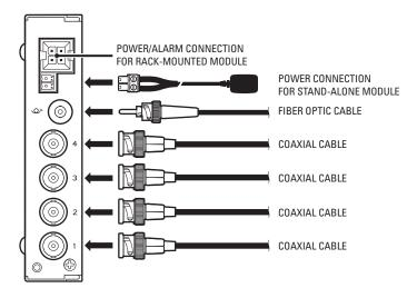
Figure 6. FT8304 Transmitter/FR8304 Receiver Connections
